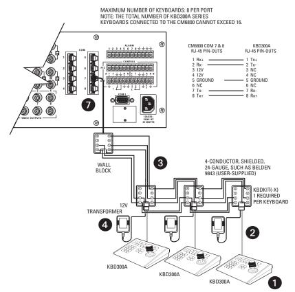
Figure 4. Connecting Remote Keyboards (CM6800-48X8 Shown)
